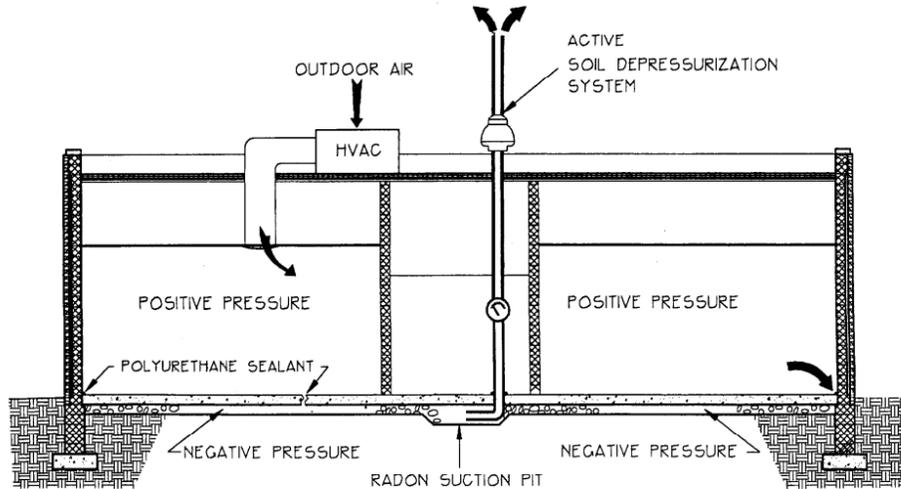
Figure 1: Illustration of the EPA Strategies for Controlling Radon Gas<sup>6</sup>
