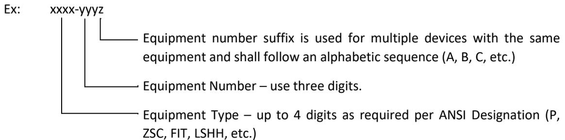
The following table lists typical tagging to be used for lift stations (pump-related tags are to be in the hundred series with the hundred's digit representing the pump number):
