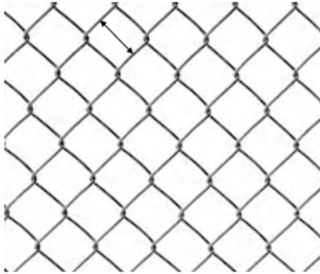
Maximum chain link mesh size and minimum gauge required for the wire core (Illustration referred to in subsection 8(3))
