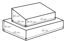
The top must be placed on the base to allow a minimum 6.3 cm (2.5") margin around the top at any point.
